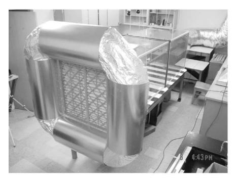
Fig. 27. Wind tunnel for assessing flight behavior of codling moth.
